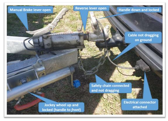
The trailer has hydraulic override brakes. When *reversing*, ensure the Reversing Stop lever is engaged to stop the trailer from auto braking.
